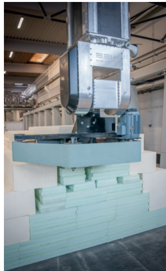
Changing from milling to grinding is possible with a simple change of the process head
