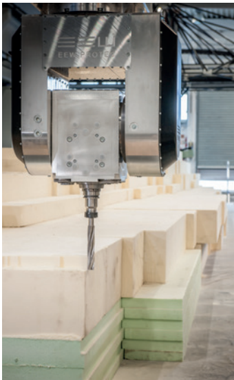
Changing from milling to grinding is possible with a simple change of the process head
